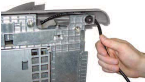
Power cable routing
